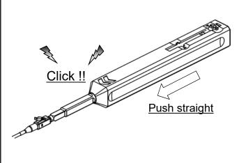
Be careful not to slant the One-Click® Cleaner LC PRO while inserting into the Adapter / Plug. Do not overly exert force during insertion as this may cause damage to both the connector and the One-Click® Cleaner LC PRO.
