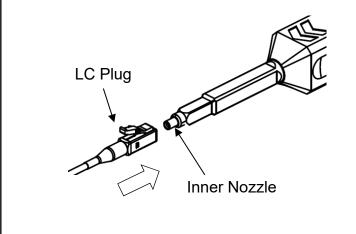
3. Push the Outer Shell to start cleaning the target connector end face. A "click" sound indicates end of cleaning process. Please attach the Dust Cap after use.
