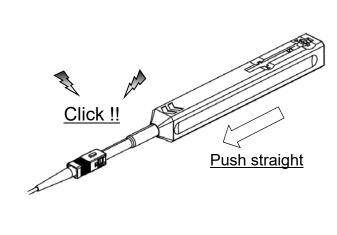
Be careful not to slant the One-Click® Cleaner SC PRO while inserting into the Adapter / Plug. Do not overly exert force during insertion as this may cause damage to both the connector and the One-Click® Cleaner SC PRO.
