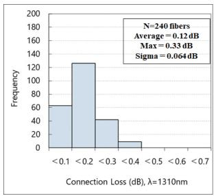
Fig. 10(a). Connection loss of hardened connector at 1310nm.
