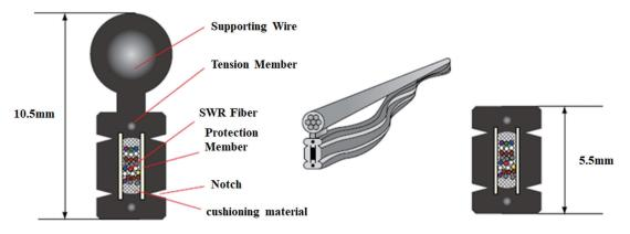
Fig. 8. 24-fiber aerial distribution optical cables <sup>5</sup>.
