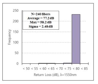
Fig. 11(b). Return loss of hardened connector at 1550nm.
