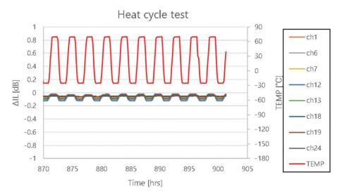
Fig. 12. Temperature cycle test results.
