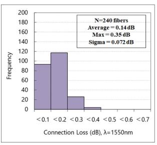
Fig. 10(b). Connection loss of hardened connector at 1550nm.
