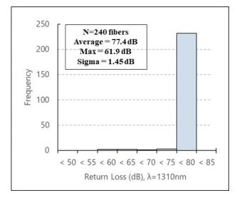
Fig. 11(a). Return loss of hardened connector at 1310nm.
